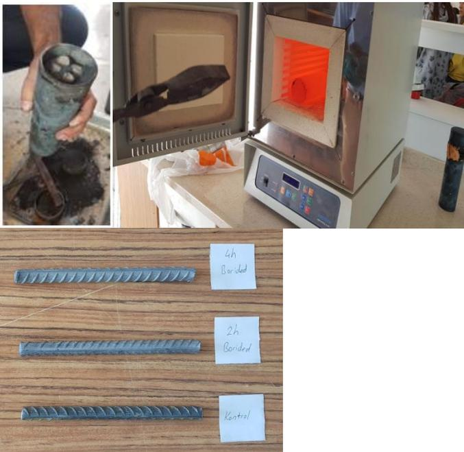
Figure 1. Coating process of rebar by boriding
