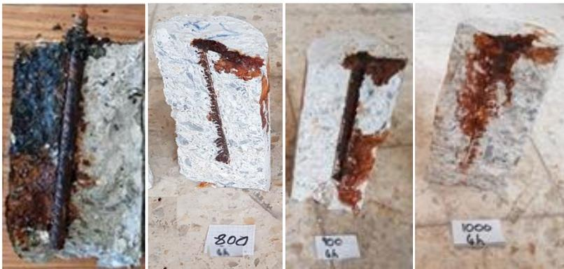
Figure 6. Inner view of corroded  $\varnothing 14$  reinforced samples depending on boriding temperature
