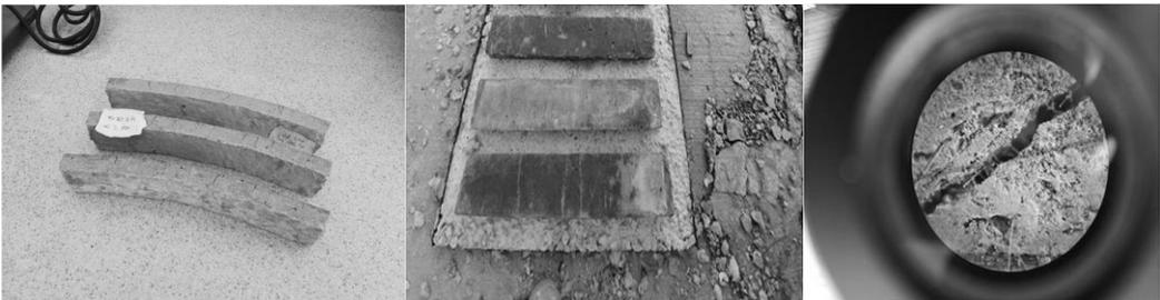
Figure 2. Small mortar beams for self-healing measurement
