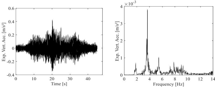
Figure 6. Mid-span vertical acceleration: experimental measurement ( $0.25 \text{ ped./m}^2$ ).
