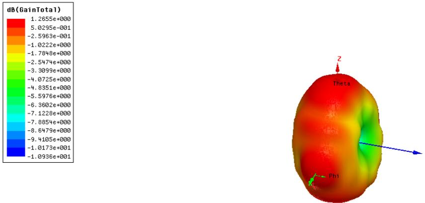
Figure 6. Gain of the patch antenna.
